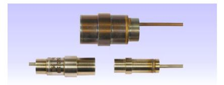
The PY non-contact displacement transducer measures the distance between its front face and a target made from a ferritic material. A ferritic material is one which is attracted by a magnet.
