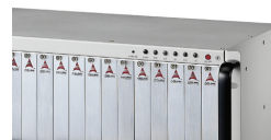
Voltage, temperature, and fan monitoring LEDs
