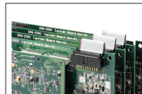
SSI bus cable for multiple cards synchronization for DAQ/DAQe-2000 series
