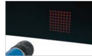
Grid 0.05 mm line thickness.
