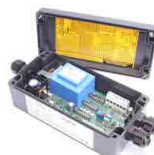
SGA Signal Conditioner/Amplifier
