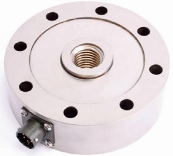
The DSCC series of pancake load cells are designed for weighing and force measurement applications and can operate in both tension and compression. They are perfectly suited for material and component fatigue testing applications where a high accuracy, low-profile device is required and forces are applied axially. The DSCC's high frequency response makes it ideal for dynamic force and load measurement applications such as crash test walls.
